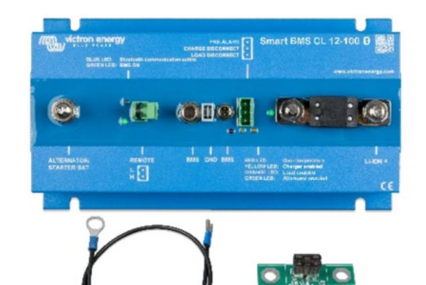
The Smart BMS CL 12-100 is an all-in-one battery management (BMS) system for <u>Victron Lithium Battery</u> <u>Smart 12,8 V</u> batteries available with a nominal voltage of 12.8 V in various capacities. This is the safest of the mainstream lithium battery types. The maximum number of batteries in one system is 20, which results in a maximum energy storage of 84 kWh in a 12 V system. It has been specifically designed for 12 V systems with a 12 V alternator such as in vehicles and boats.
