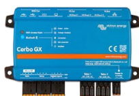
Ekran GX or Cerbo GX Provides intuitive system control and monitoring and enables access to our free remote monitoring website: the VRM Online Portal.
