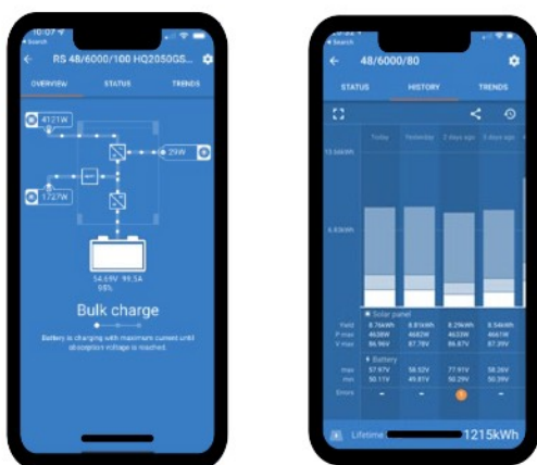
Configure and monitor with VictronConnect A built in Bluetooth Smart connection allows for quick monitoring or settings adjustment of the Multi RS.
